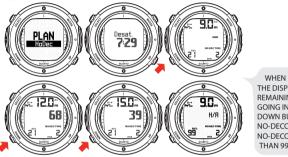
WHEN ENTERING THE PLAN MODE THE DISPLAY FIRST BRIEFLY SHOWS THE REMAINING DESATURATION TIME BEFORE GOING INTO PLAN MODE. USE UP AND DOWN BUTTONS TO SCROLL DIFFERENT NO-DECOMPRESSION LIMITS. NO-DECOMPRESSION LIMITS. NO-DECOMPRESSION LIMITS LONGER THAN 99 MINUTES ARE DISPLAYED AS "-"
